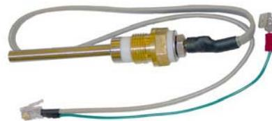
**CAUTION:** Do not use plumber’s tape/Teflon tape/pipe dope when installing the P65 Thermowell. Tape will prevent the low water detection system from operating properly and will cause false low water errors. Lubricate O-ring prior to installation. Tighten probe at the brass hex flats only.
