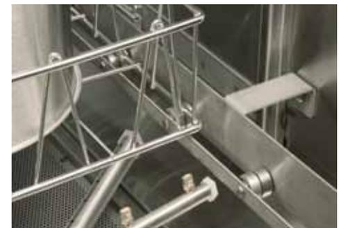
Rollers make getting large racks in and out of the pot washer easier. Available on the CA-3 and DA-3 models.
