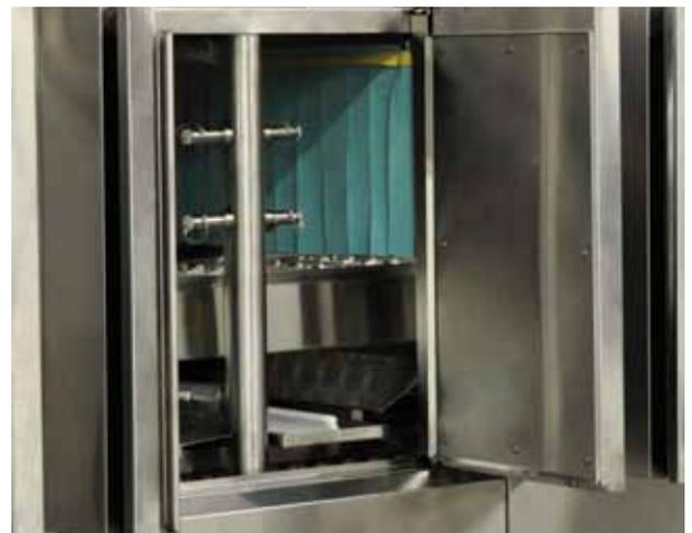
Swing Doors provide wide access into the interior of the machine. Paired with the standard overhead interior lights, daily maintenance and service is quick and efficient.
